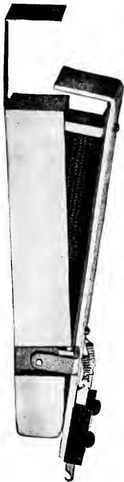
FIG. 162.—Western Rising Visual Signal for use on central energy switchboards. The magnet coil is energized by a direct current battery after the circuit has been made with the subscriber, and the target remains raised until the plug is inserted in the cut-out jack.
